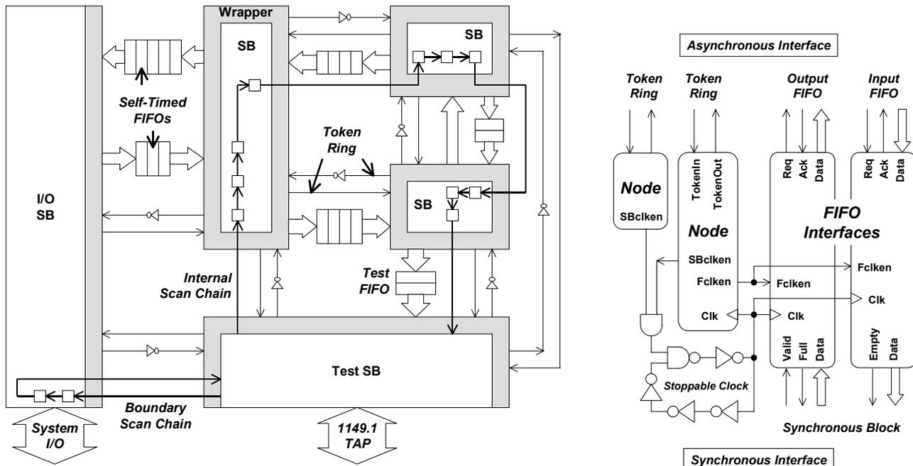
Figure 1: A. Synchro-tokens system architecture.
